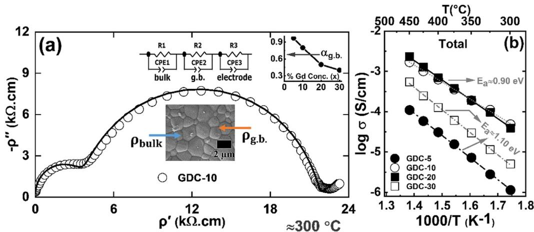
Fig. 1. (a) Illustration of a characteristic impedance spectrum of GDC-10 sample, measured at 300 °C in air with silver (Ag) electrode. The inset plot shows the relation of the ion-blocking factor as a function of dopant concentration. (b) The Arrhenius plot for the estimation of total electrical conductivities of the sintered GDC pellets.
