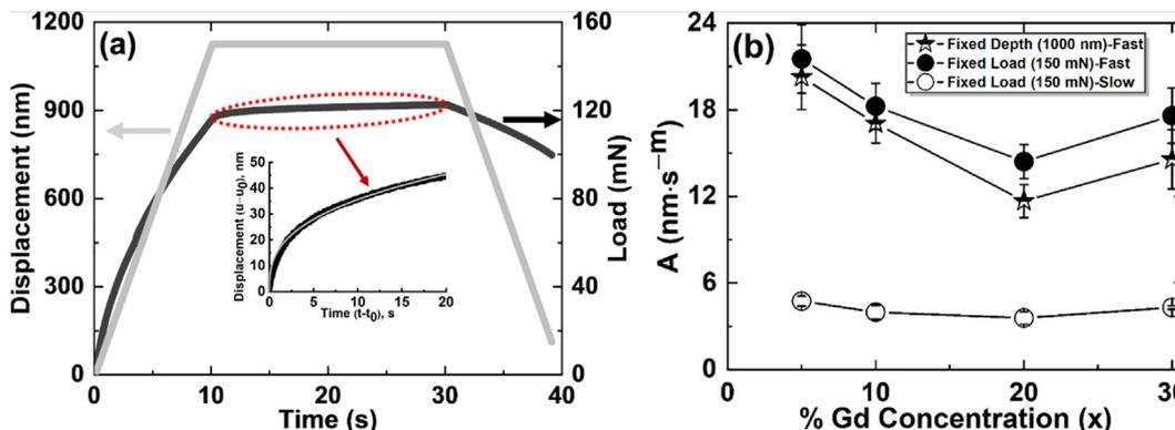
Fig. 2. (a) The representative load-time and displacement-time curve of a GDC-10 sample in the nanoindentation fast loading approach. The inset shows a non-linear displacement-time plot in the holding segment, indicating a primary creep. (b) The creep constant (A) as a function of Gd-doping in ceria compositions under fixed depth (fast) and fixed load (fast/slow) mode.
