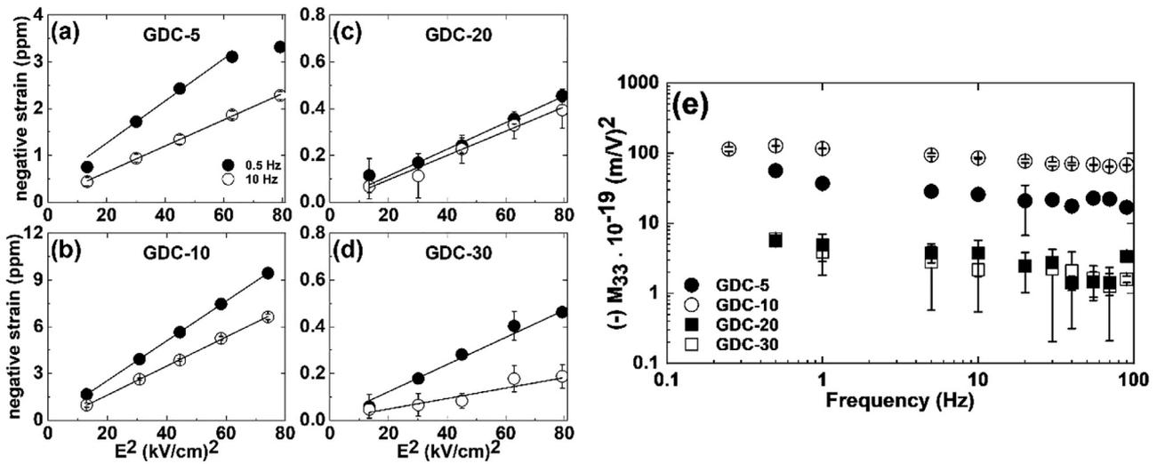
**Fig. 3.** (a–d) The electrostrictive negative strain with the response to the external electric field at frequencies 0.5 and 10 Hz for GDC samples (Gd = 0.05–0.3), electrode material: Gold (Au). (e) The electrostrictive strain coefficient ( $M_{33}$ ) as a function of frequencies ranging from 0.15–100 Hz.
